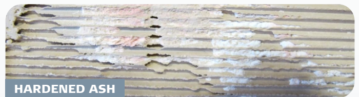
Cut-through of a filter after it went through a 2-stage cleaning. The white residues remains, and will continue to partially block the exhaust flow.
