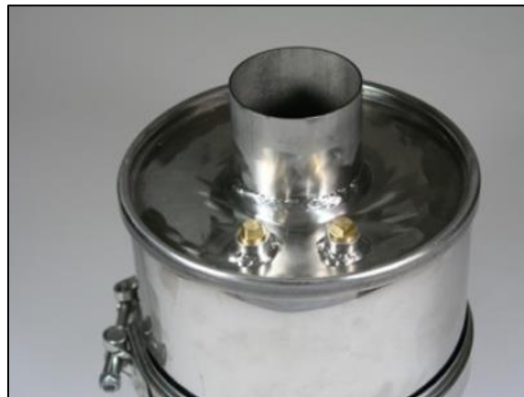
Figure 2.11. DPF pressure and temperature monitoring points for a \frac{1}{4} NPT fittings
