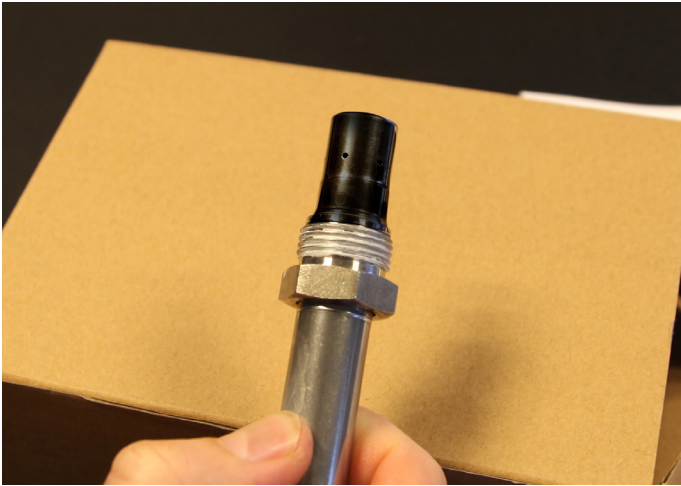
Figure 12. Evidence of excessive soot/ash.
