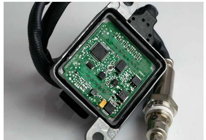
Figure 3. Sensor circuit board
