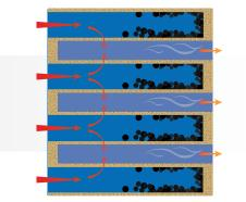
Regeneration (regen) requires high exhaust temperatures of 570°-750°C. Combining high temperatures and a unique mix of precious metals washcoat and substrate turns soot into ash. The DPF is now regenerated and ready for use.
