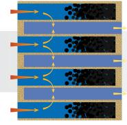
Over time, soot builds up in the DPF. Eventually, this causes backpressure detected by the Engine Control Unit (ECU) necessitating regeneration.
