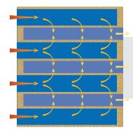
Exhaust gasses containing soot enter the DPF. The filter traps any matter larger than one micron, allowing gasses through.
