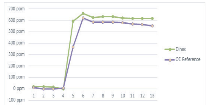
Test of Dinex vs. OE sensors, showing equal accuracy.
