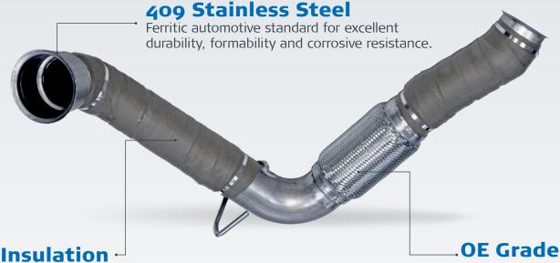
Several insulation techniques available to ensure proper heat retention for pipes & aftertreatment systems.
