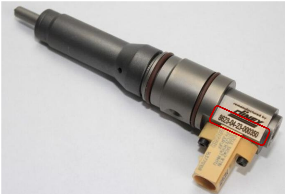
Fig. 1. Traceability code printed on the injector
