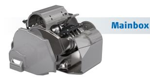
At first the Mainbox may seem similar to a Euro 7 aftertreatment system as the wellknown the key catalyst functions are present; Diesel Oxidation Catalyst (DOC), Diesel Particulate Filter (DPF) and SCR catalyst including injection and mixing of Urea. But from there, the resemblance stops. If not included in the Prebox, the Mainbox also contain the first of two SCR catalysts in front of the DOC.
