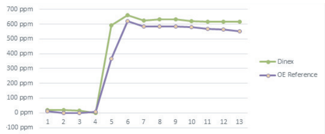
Test of Dinex vs. OE sensors, showing equal accuracy.
