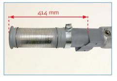
**Step 3**: Make sure that there is 414 mm (+/- 2 mm) distance between the clamp and the pipe end.
