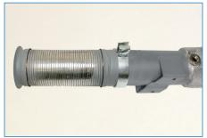
**Step 4**: Secure the clamp by tightening the bolt.
