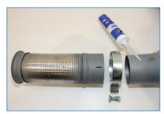
**Step 2**: Before connecting the pipes uniformly, apply Dinex Exhaust Assembly Paste (78800).
