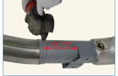
**Step 1**: Cut the pipe as close as possible to the flex hose and make sure that it is not less than 139 mm from the bracket.
