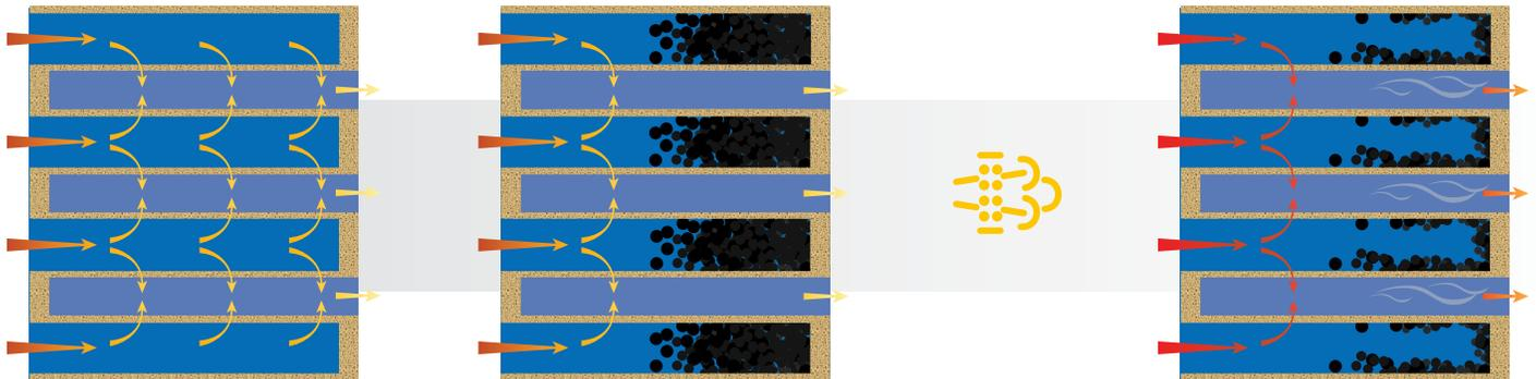
Exhaust gasses containing soot enter the DPF. The filter traps any matter larger than one micron, allowing gasses through.
